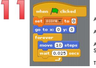
Add a forever loop Add a move 10 steps motion block Add a wait control block Set the value to 0.025 secs
